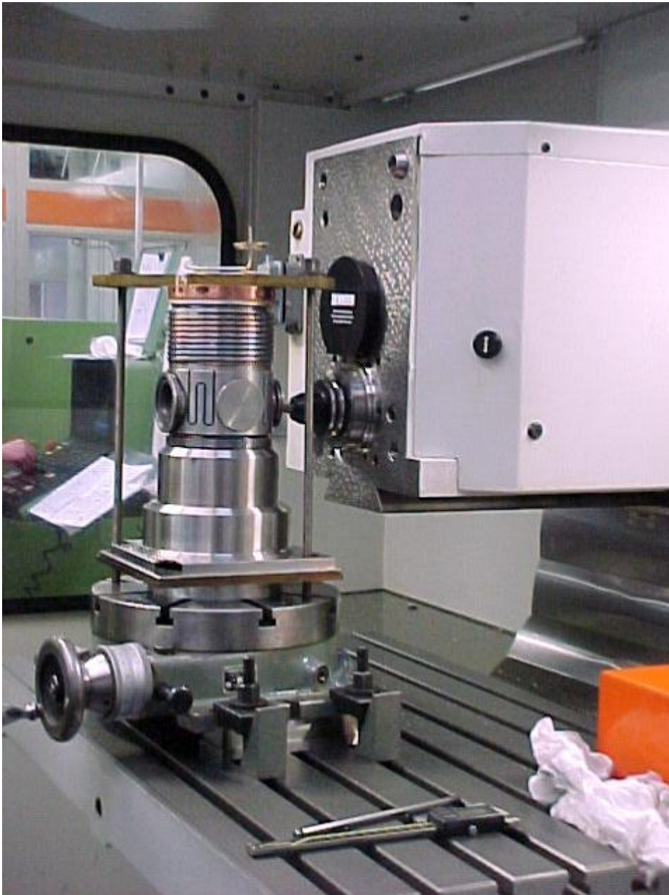
Figure 9. The HTI (High Temperature Insert) during manufacturing at the University of Amsterdam; this insert will be used to study water at 373°C.
