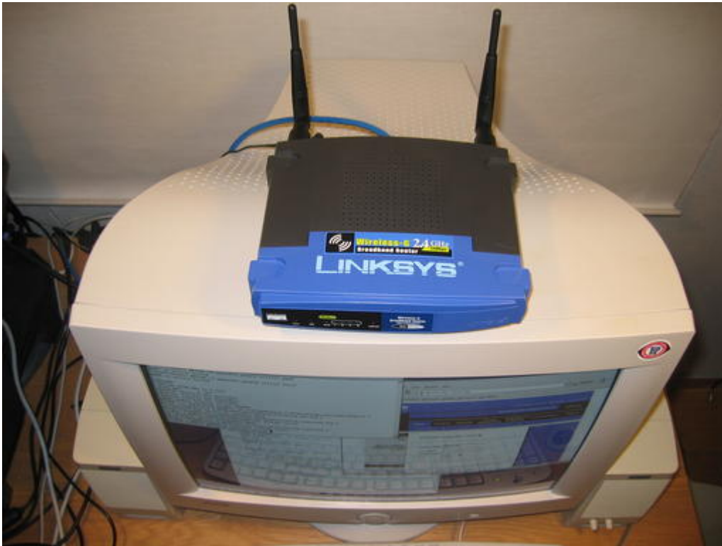
Figure 1. For under $100 US, the Linksys WRT54G is a capable Linux platform with 16MB of RAM, a 125MHz processor and support for 802.11b and g.
